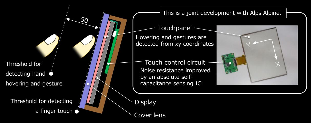
• Two-step operation, non-touch and touch interactions, can be detected based on capacitance
