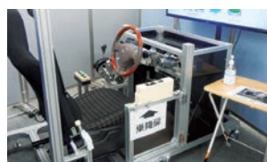
A mock-up that allows you to experience product defects from the customer's perspective
