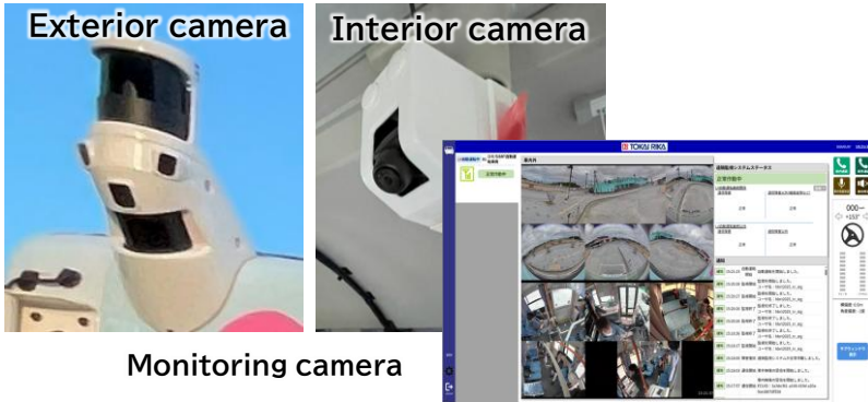
Example of remote monitoring system
