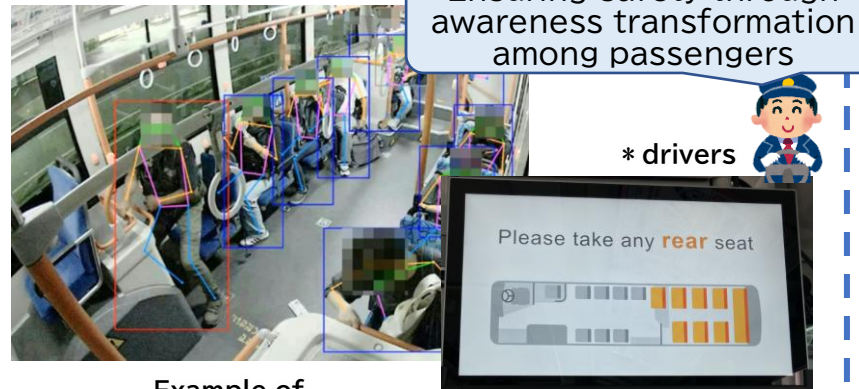
Example of AI-based human detection and pose estimation Passenger guidance display (seat availability guidance)
