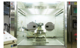
温度条件下のターンキャンセル評価 Evaluation of turn switch cancellation under various temperature conditions
