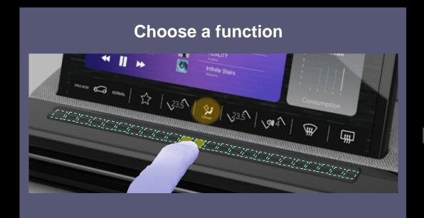
The capacitive sensor in the knob detects the position of a finger.
