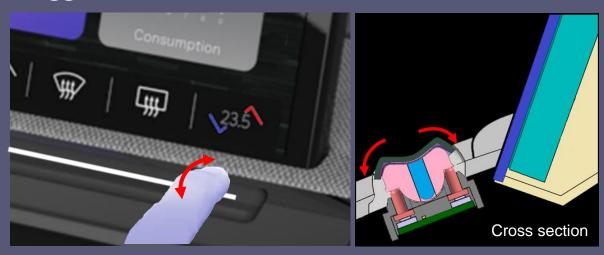
A toggle switch is suitable for temperature control or other up-and-down operations.
