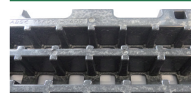
Disposed due to dirt that cannot be removed by air blow
