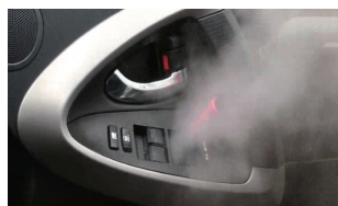
Window regulator switch steam cleaning test
