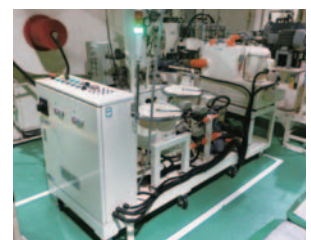
▲静電浄油機と遠心分離機 Electrostatic oil purifier and centrifuge
