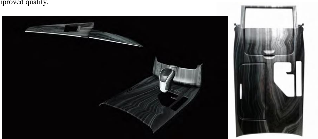
Automobile interior panels decorated using the 3D dry transfer method
